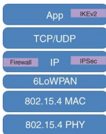
Figure 3.39 IP stack on smart meter with 6LoWPAN, firewall, and IPSec-IKEv2 on ZigBee SoC
