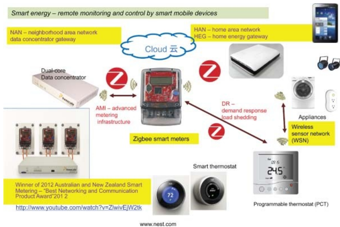
Figure 3.14 Smart grid with smart meter, HAN, and NAN
